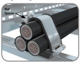
**6.** Using supplied mouthpiece fittings, tighten down to no more than 8Nm with 19mm nut spanner.
