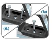
**3.** Secure cleat to the mounting surface using 1x M10 bolt (3a) or 2 x M10 bolts (3b), adding a washing and nut on both sides.
